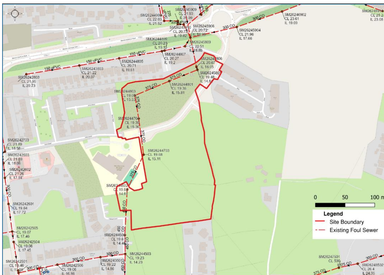
Figure 4-1: Existing Foul Sewer Network at Project Site. Source (QGIS)
